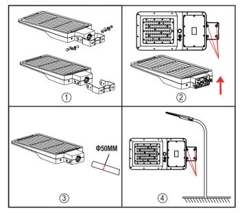
Loosen the screws and remove the big U-shaped bracket.
